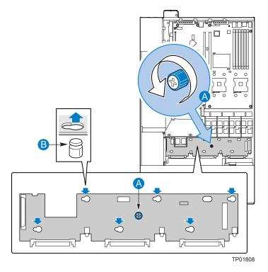
Figure 47. Removing the SATA or SCSI Backplane from the Chassis
